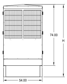
All enclosure models are 200 MPH wind rating certified in accordance with IBC2018 and ASCE/SEI 7-16 standards.
